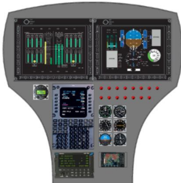
Figure 23: Main Control Panel
